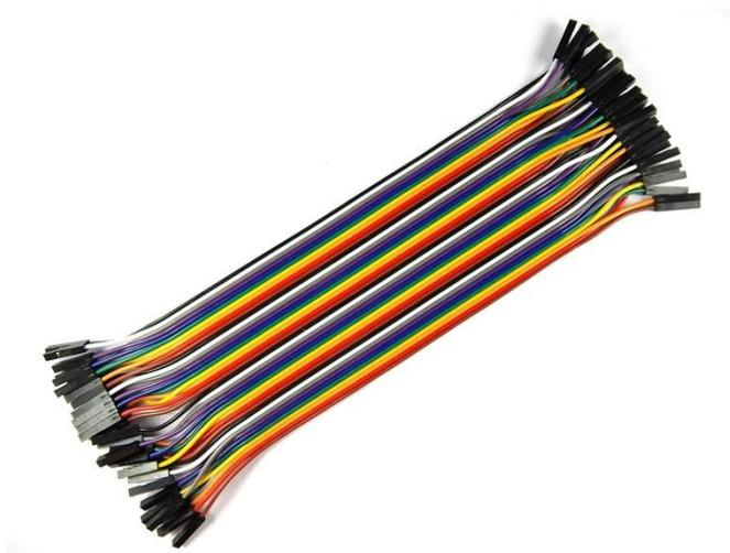
Fig. 5. Jumper Wire
