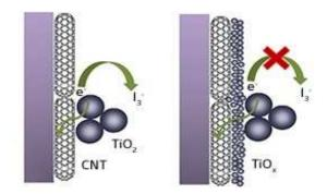
In earlier designs (left), the carbon nanotubes degraded through chemical processes (e-: electrons, I3-: ions in the liquid). Using a thin protective layer of titanium oxide now stabilizes the nanotubes (right), increasing the performance of these cells. It uses low-cost organic dyes and titanium dioxide (TiO2) nanoparticles in place of expensive semiconductor and rare earth elements to absorb sunlight.
