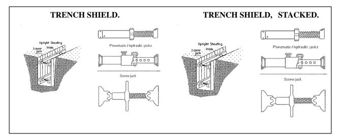
**COMBINED USE**. Trench boxes are generally used in open areas, but they also may be used in combination with sloping and benching. The box should extend at least 18 in (0.45 m) above the surrounding area if there is sloping toward excavation. This can be accomplished by providing a benched area adjacent to the box.
